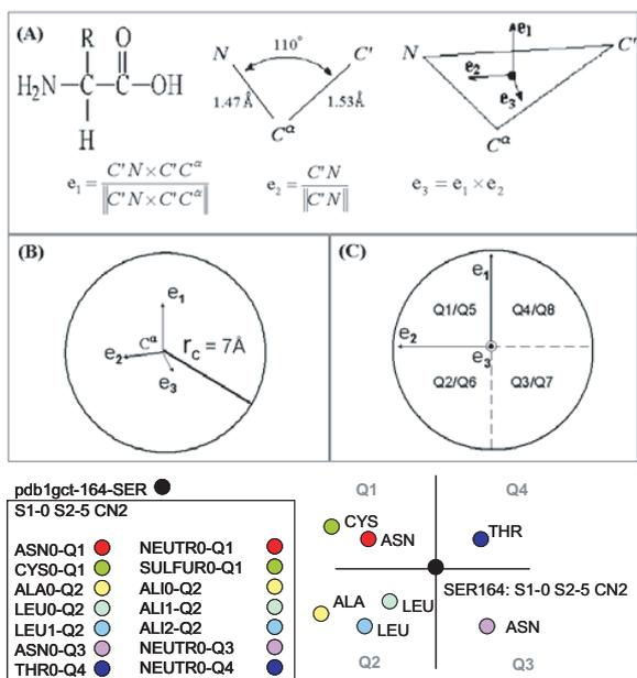
**Fig. 2.** Feature extraction methodology. (A) Definition of residue-centered reference-frame. (B) Examination of microenvironment, and the type and identity of residues in the geometric subspaces Q1–Q8 and (C) the results for Ser-164, in S1 subfamily.
